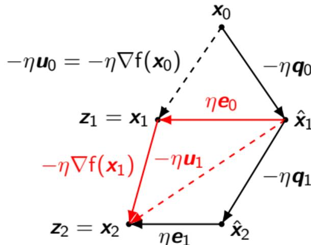
Differential quantization<sup>1</sup> directs the quantized trajectory to the unquantized trajectory.
